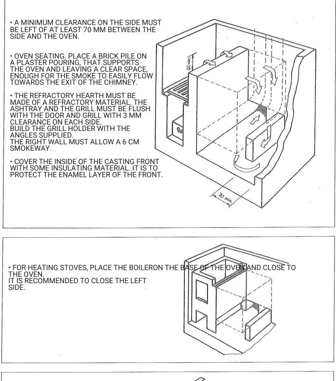
• ANCHORING OF THE FRONT. PLACE THE FRONT ANCHOR ON THE BUILDING SITE AND FASTEN IT THE FOUR ANCHORS, MAKE THE BASE MATCH THE ASHTRAY DOOR AND THE SMALL DOOR. IN THE MODELS WITH A DOOR PANEL, FILL THE GAP BETWEEN THE FRONT AND THE BOILER WITH SAND, PLASTER OR OTHER OR OTHER INSULATING MATERIAL.
